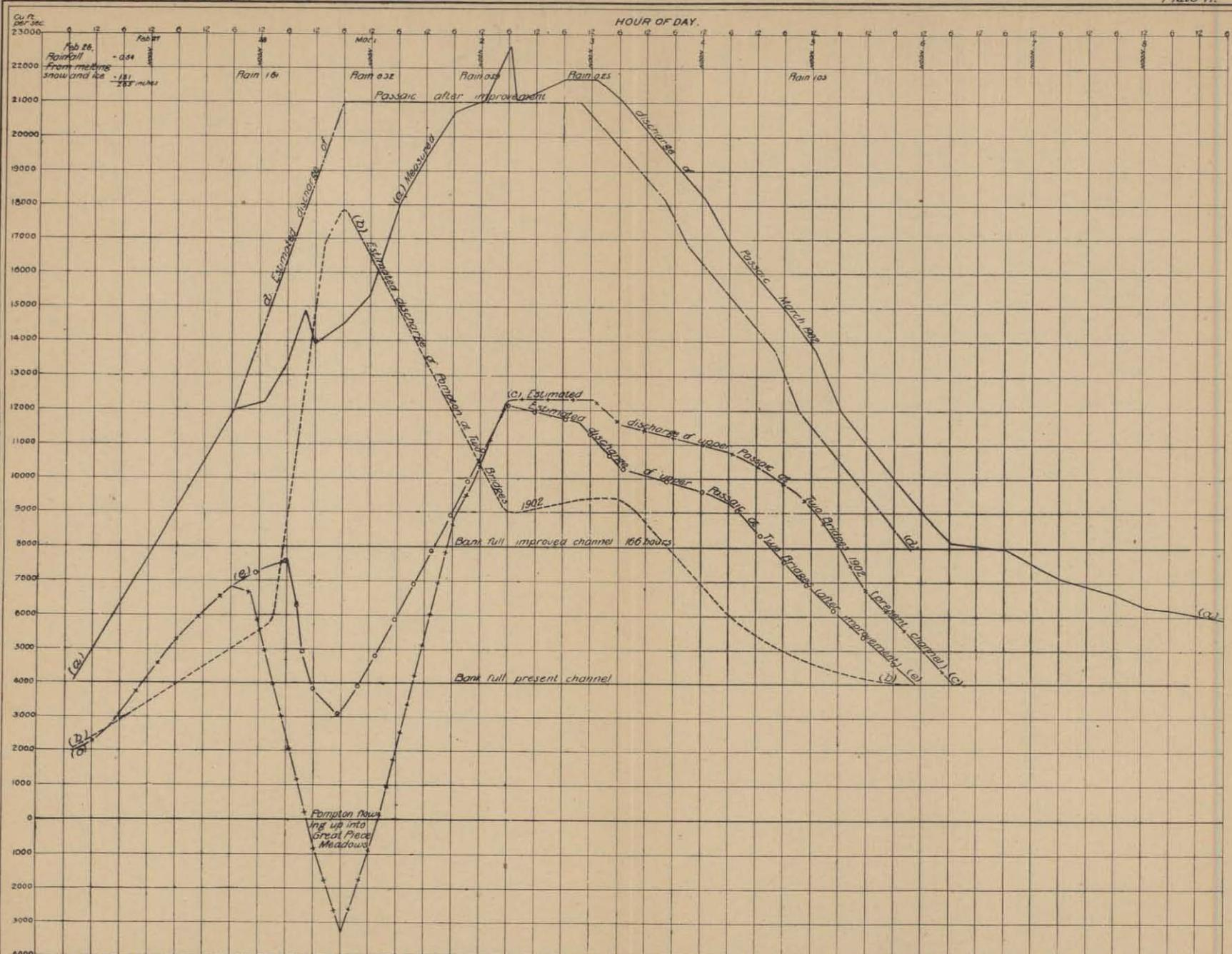
DIAGRAM SHOWING MEASURED FLOW OF PASSAIC RIVER FEB. 27<sup>th</sup> TO MAR. 9<sup>th</sup> 1902 AND THE ESTIMATED FLOW OF ITS TWO TRIBUTARIES AT TWO BRIDGES. ALSO ESTIMATED FLOW OF THE PASSAIC AFTER COMPLETION OF PROPOSED DRAINAGE WORKS ABOVE LITTLE FALLS.
