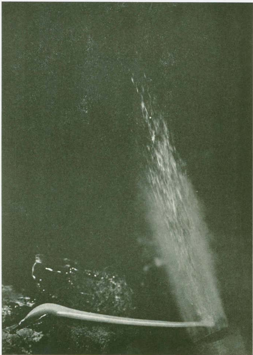
FIGURE 9. The Blowing of mineral wool. (Courtesy of Baldwin-Hill Company, Trenton, New Jersey.)
