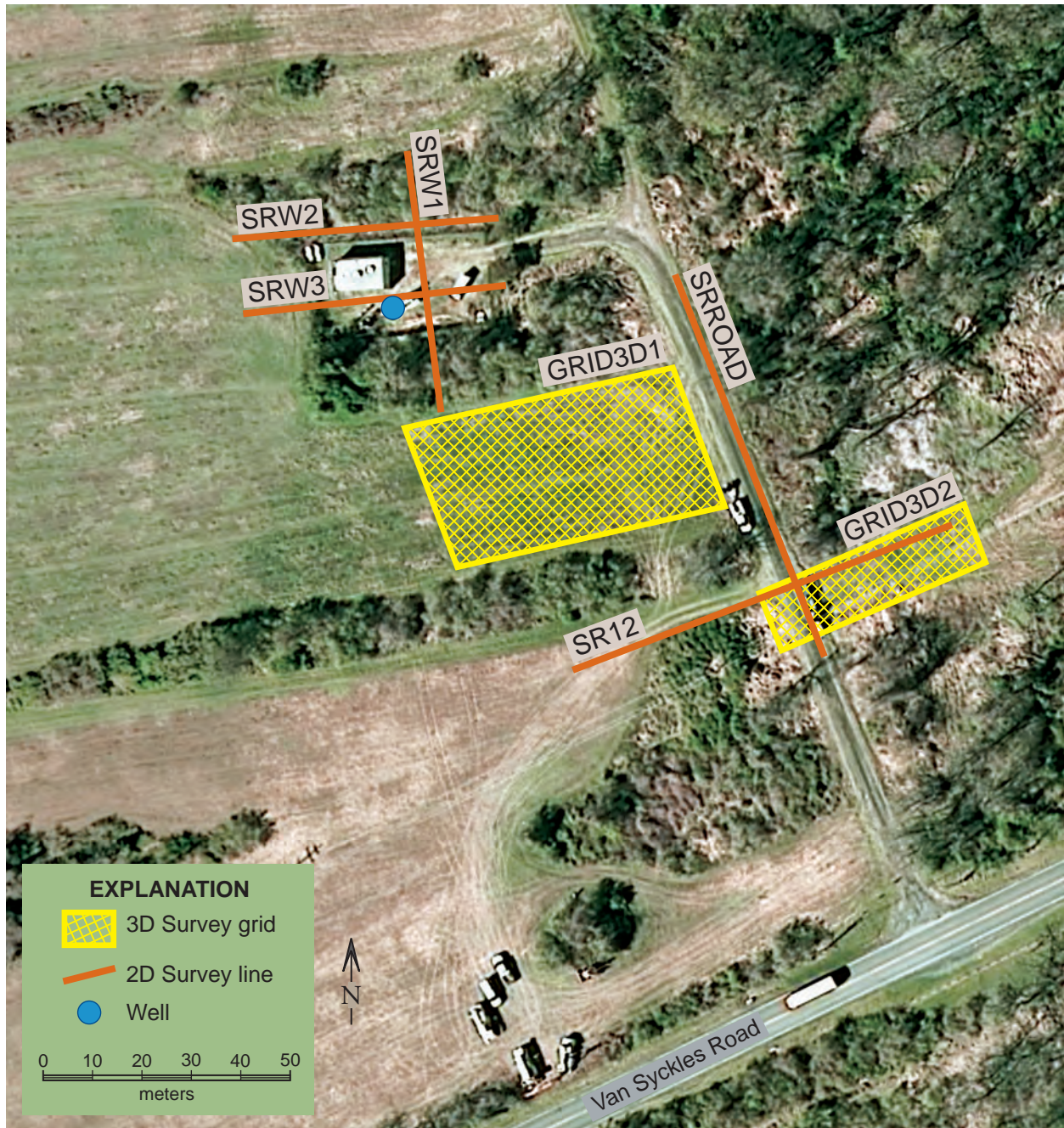
Figure 4. Locations of the electrical resistivity survey lines and grids. Aerial photo: NJ Department of Environmental Protection.
