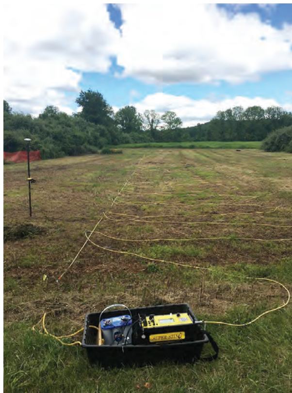
Figure 6. The AGI SuperSting R8/IP™ resistivity meter connected to a 12 V battery and a 28-electrode multicore cable collecting a 2D resistivity profile. The cable is connected to stainless steel electrodes pushed into the sub-surface. The Trimble Geo 7X GPS unit shown on the left side of the figure. Photo by M. Gagliano.
