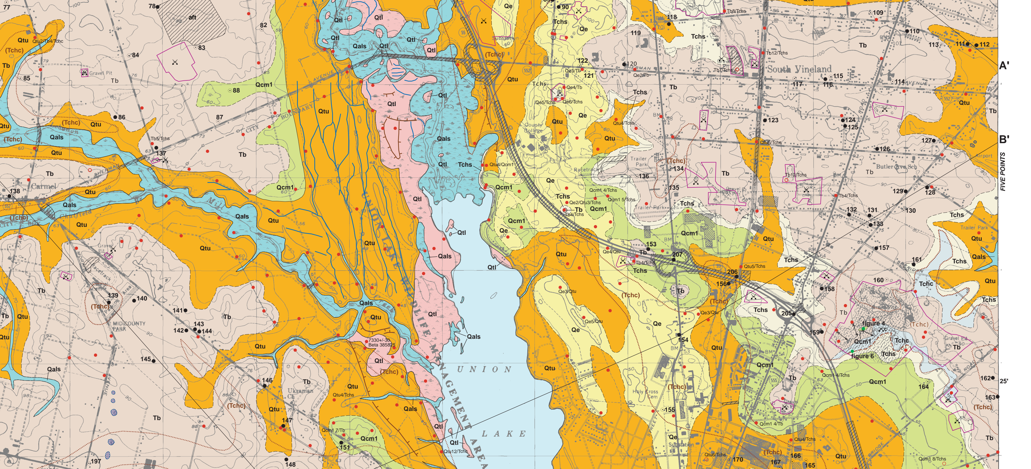
Figure 2.—Surficial deposits and geomorphic features of the Millville quadrangle. The upper stream-terrace deposits in a valley cut into the Bridgton fluvial plain during the early and middle Pleistocene. The lower stream-terrace deposits and modern floodplains are in inner valleys eroded into the upper terrace during the Wisconsinan glacial stages of the late Pleistocene. The Cape May 1 deposits were laid down during a sea-level highstand in the middle Pleistocene.
