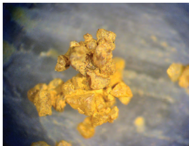
Figure 2. Photomicrograph of a quartz sand aggregate cemented with jarosite from the Merchantville Formation at Cheesequake State Park. 50 times magnification.
