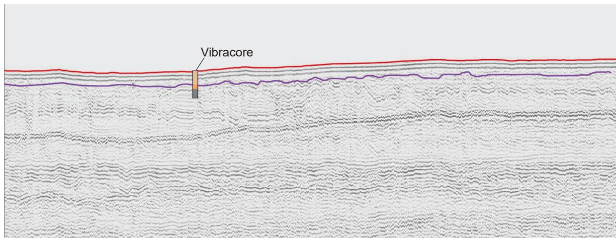
**Figure 5.** Seismic profile showing the traced seafloor (red), a vibracore with sand (tan) in the top layer, and the tracing of the base of the sheet sand layer (purple).
