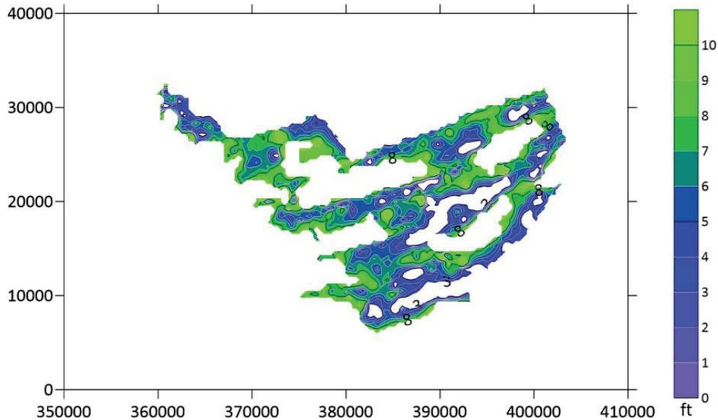
**Figure 7.** Isopach map of the Cape May sheet sand area showing where the sheet sands are greater than 3 feet thick.
