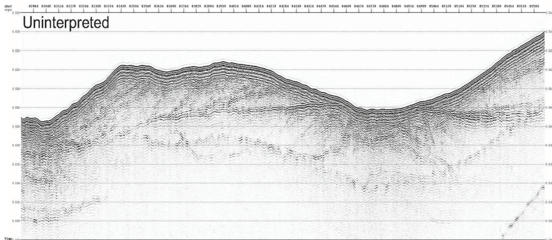
**Figure 2.** Digital seismic profile showing the seafloor and the stratigraphy of the underlying sediment layers.
