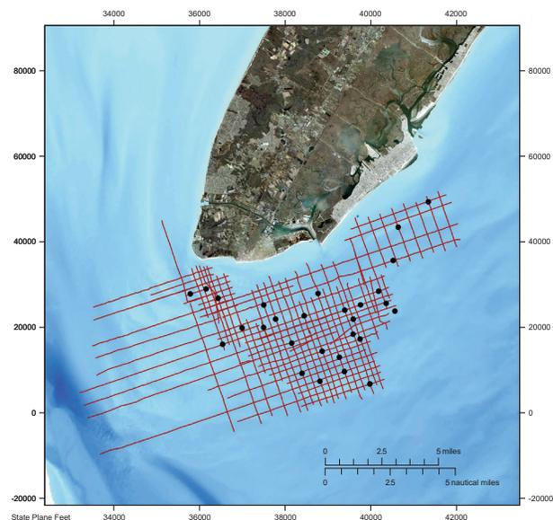
**Figure 1.** Seismic data (red lines) and vibracores (black dots) previously collected by the New Jersey Geological and Water Survey in 2003 and 2005. Data was chosen due to the closer than normal spacing and high quality.
