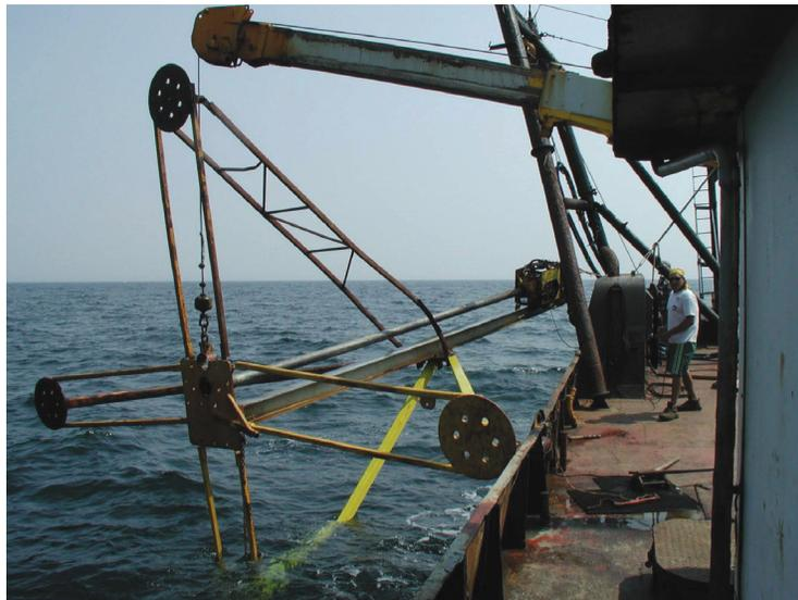
**Figure 3.** Vibracore rig onboard vessel. The A-frame and core barrel are lowered to rest on the seafloor. The motor on the top of the A-frame is then vibrated pushing the core barrel and into the sediments to retrieve a relatively undisturbed sediment sample. *Photo by J. Uptegrove*
