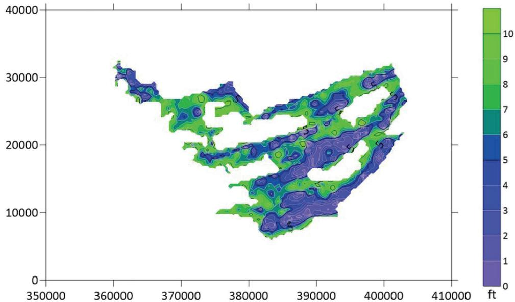
**Figure 6.** Isopach map of the Cape May sheet sand area showing all sand to the base of the sand shoal.
