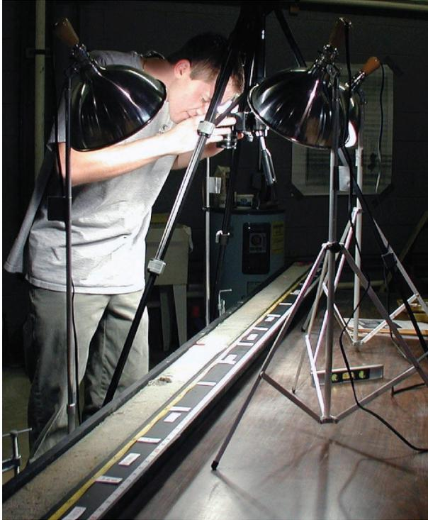
**Figure 4.** Laboratory work on the vibracoe samples includes photographing, sampling of the sediments, and grain size analyses. *Photo by J. Uptegrove*
