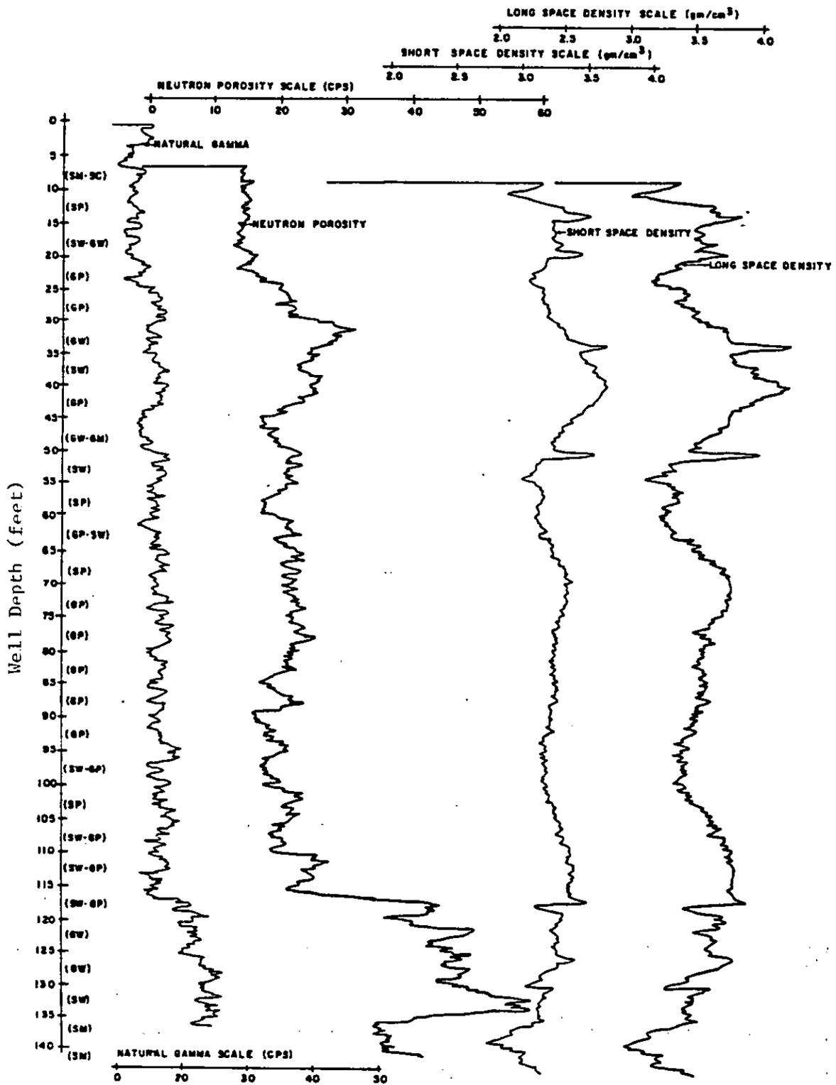
Geophysical logs of Test Well TW-5.
