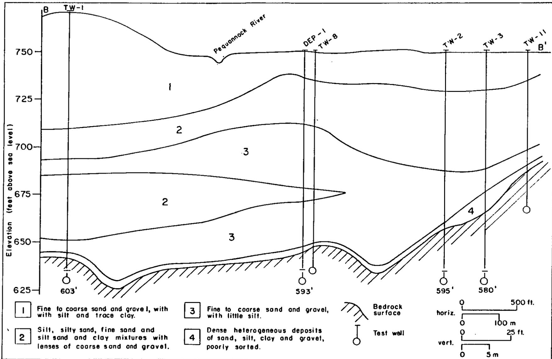
Figure 4. Cross section of valley fill deposits along the Pequannock River in Area 1, Jefferson and Rockaway Townships.
