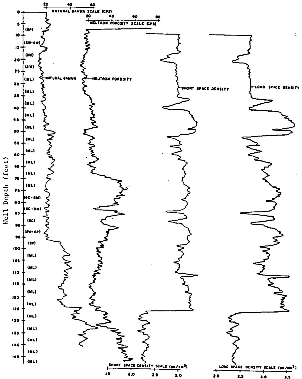
Geophysical logs of Test Well TW-2.
