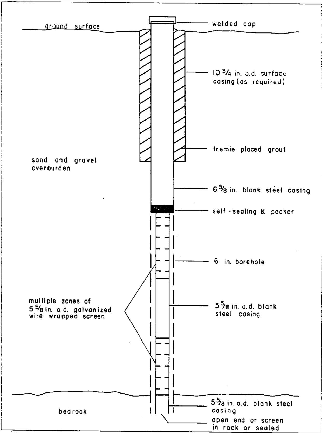
Figure 11. Construction of test wells used in the study.
