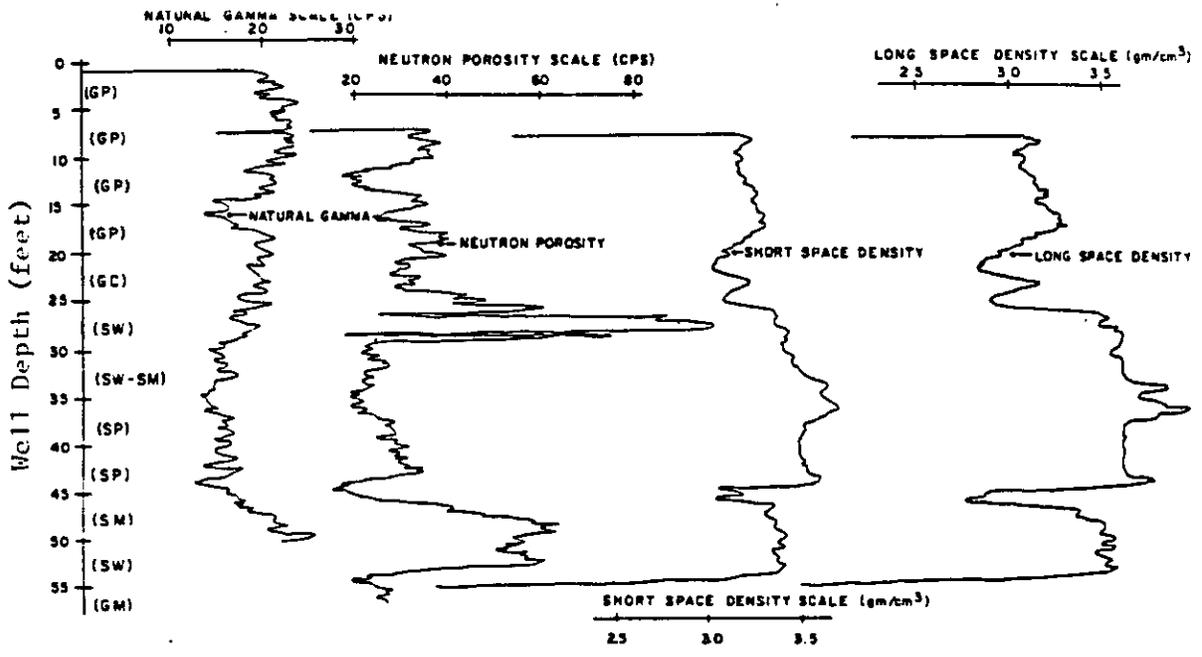
Geophysical logs of Test Well TW-11.
