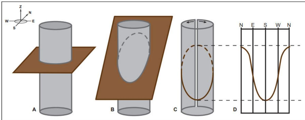
**Figure 14.** “Unrolling” OPTV data diagram. (A) gently-inclined plane intersects the borehole wall creating a low amplitude cut, whereas, (B) a steeply-inclined plane intersects the borehole wall creating a high amplitude cut and (C) trace. (D) the steeply-inclined trace “unrolled” shows a high amplitude curve with a steep dip to the south (Beetle-Moorcroft, 2018).
