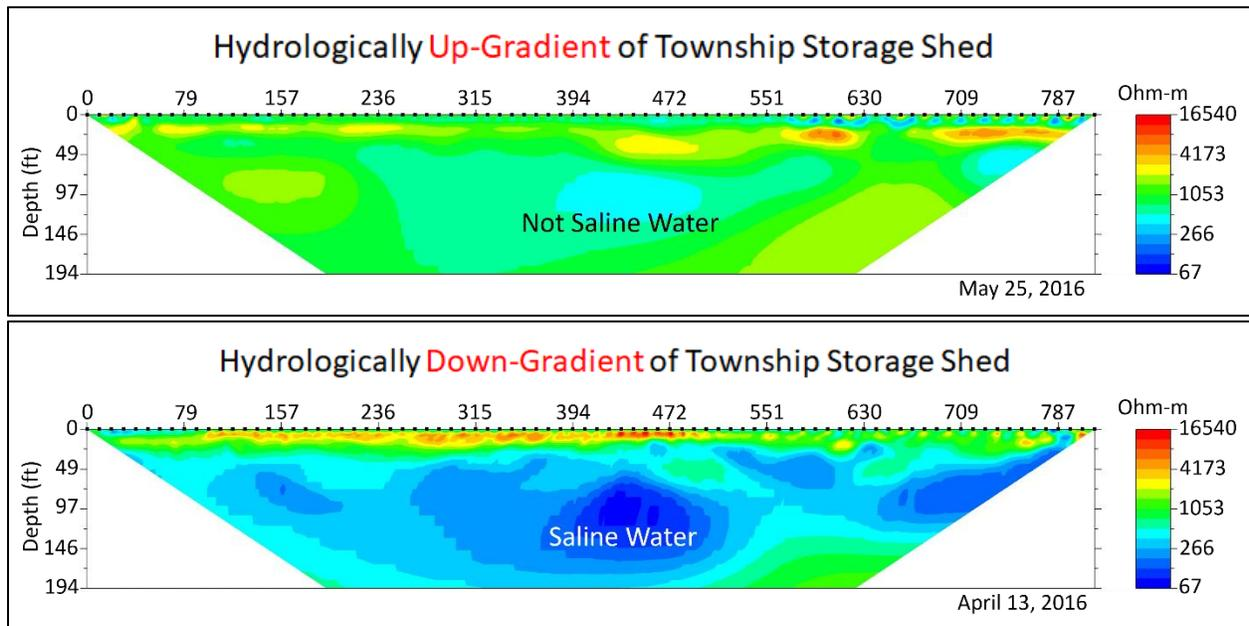
**Figure 21.** Surface Resistivity Results Up-gradient and Down-gradient of Knowlton Storage Shed.
