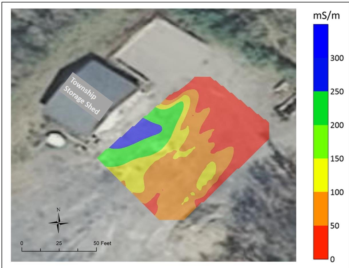
**Figure 22.** Electromagnetic Survey Adjacent to Knowlton Township Storage Shed, millisiemens per meter (mS/m).
