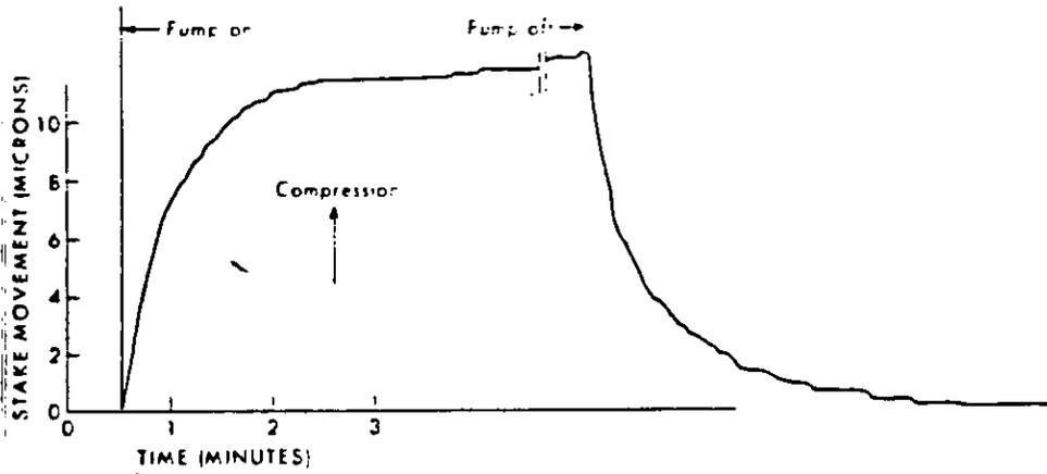
Tracing of a strip chart recording showing typical relative movement of the stakes to one cycle of starting and stopping the pump.
