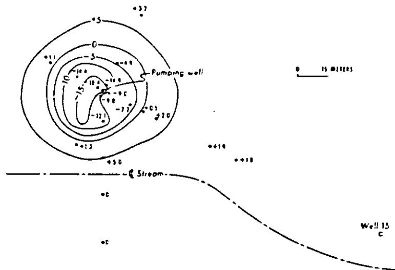
Contour map of radial strains, measured at the surface, as a result of starting pumping. —, posts moving together; +, posts moving apart; contours, strain  $\times 10^{-4}$ .
