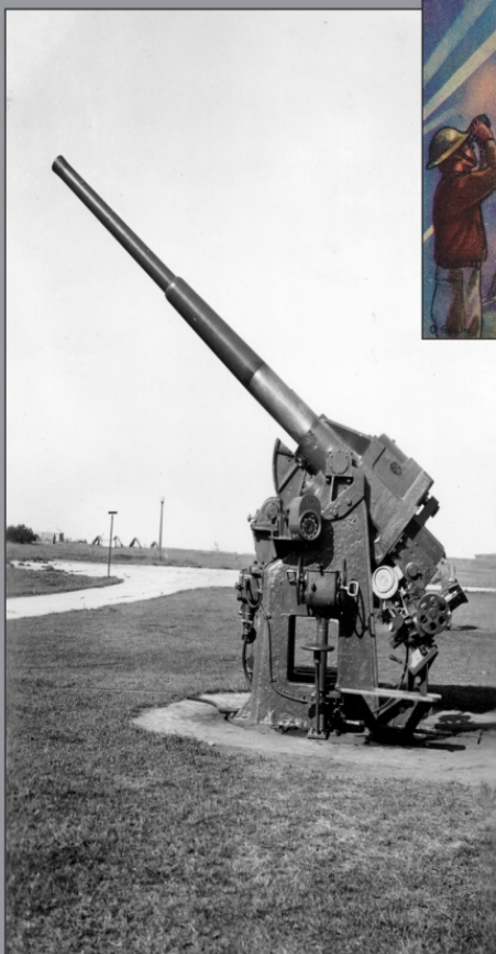
3 inch anti-aircraft gun on M1917 pedestal mount - Coastal Defense Study Group
