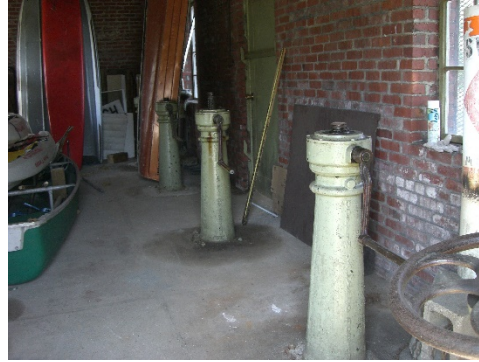
Hand cranks control sluice gates and fountain
