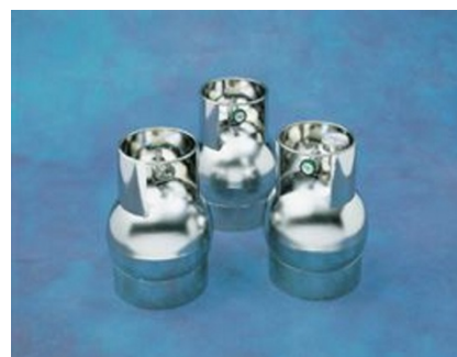
Typical air sampling canister
