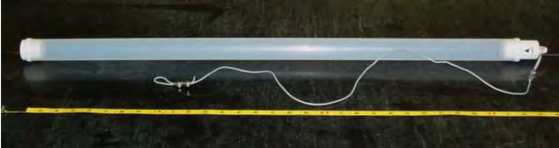
Figure 5.1 Bottom fill bailer with Teflon® coated stainless leader (Photograph by J. Schoenleber)
