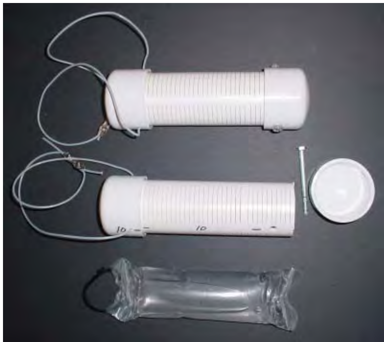
Figure 5.16 PDB for Sediments using bag provided by Columbia. (Photograph by J. Schoenleber)
