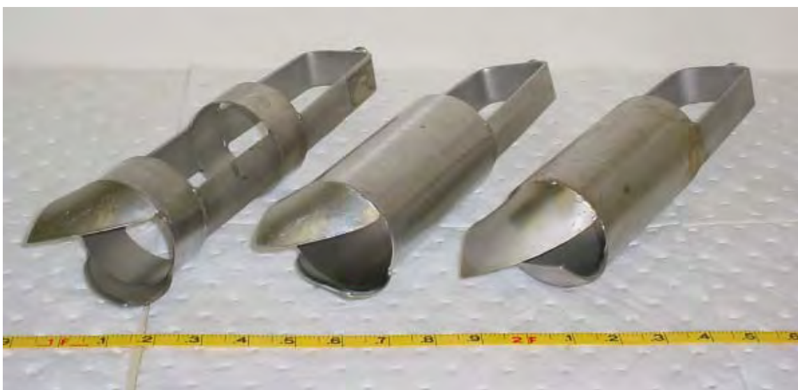
Figure 5.32 Bucket Augers (Photograph by D. Dibblee)
