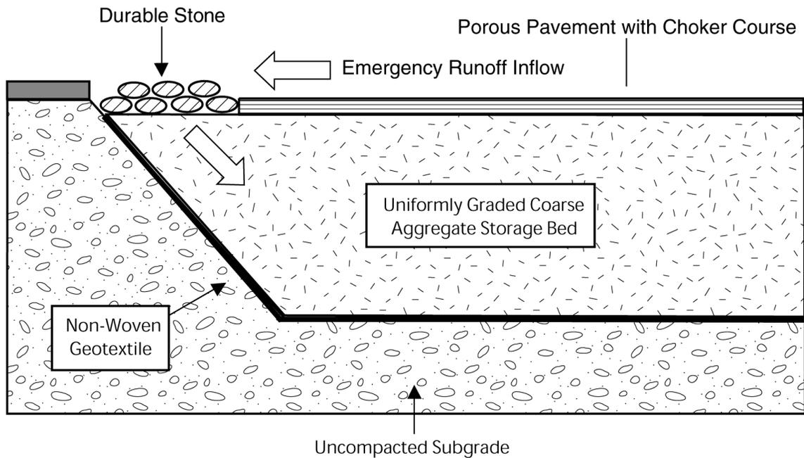
Note: Emergency inflow may also be provided by surface drain inlets and perforated pipes in the storage bed. See text for details.
