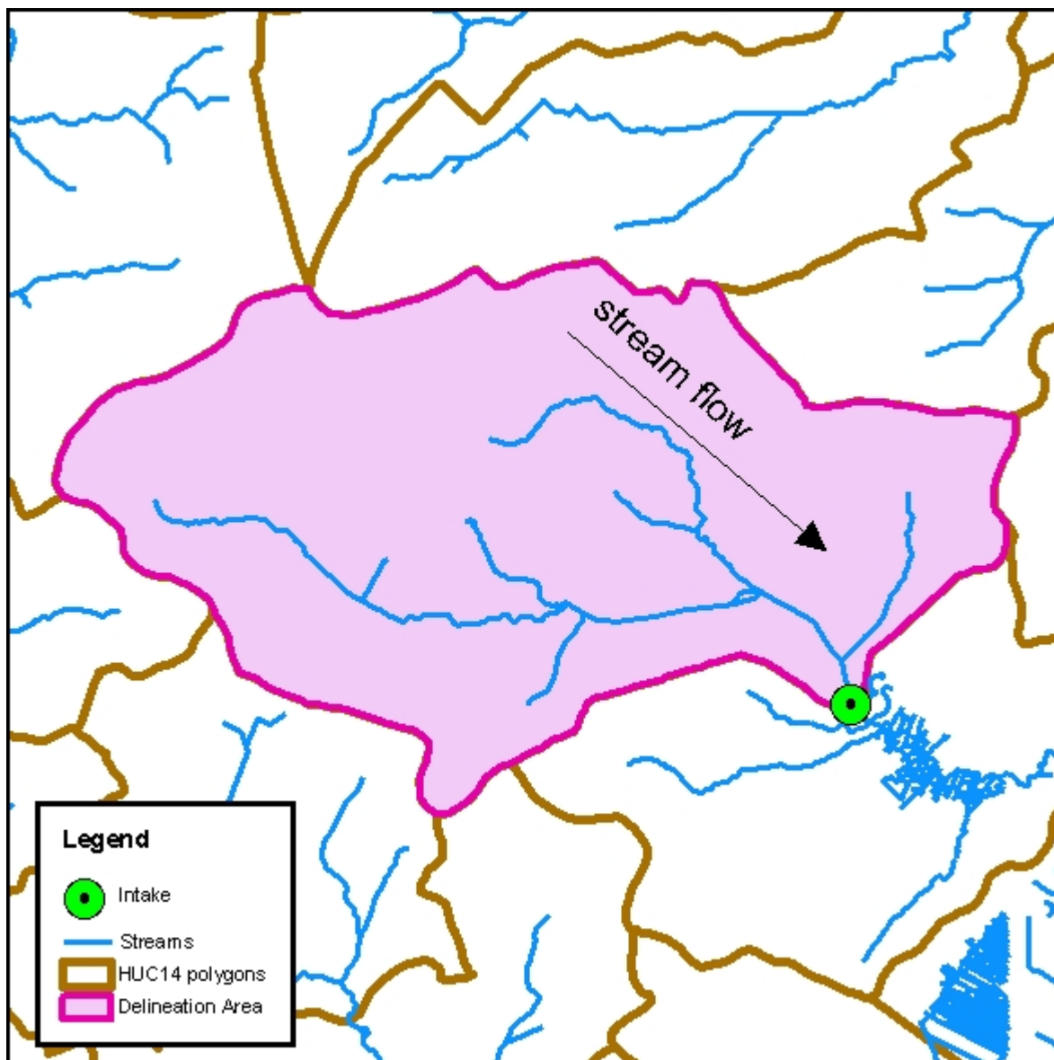
Figure 3. Example of delineated contributing area to a water-supply intake.
