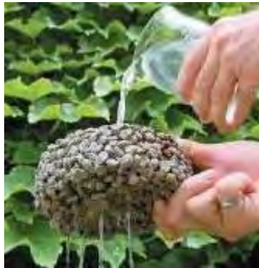
Figure 7.2: Example of pervious concrete allowing water to flow through it 1
