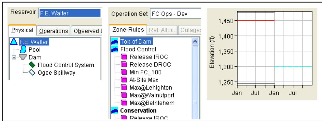
Figure 4.34 F.E. Walter's Pool and Dam Elements and its "operating zones" and rules
