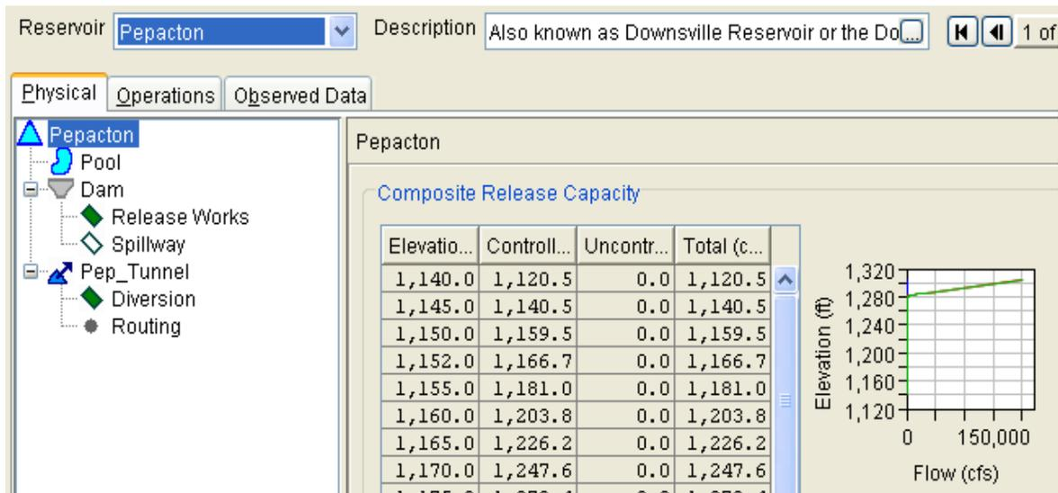
**Figure 4.18** Pepacton Physical Element Tree and Composite Release Capacity
