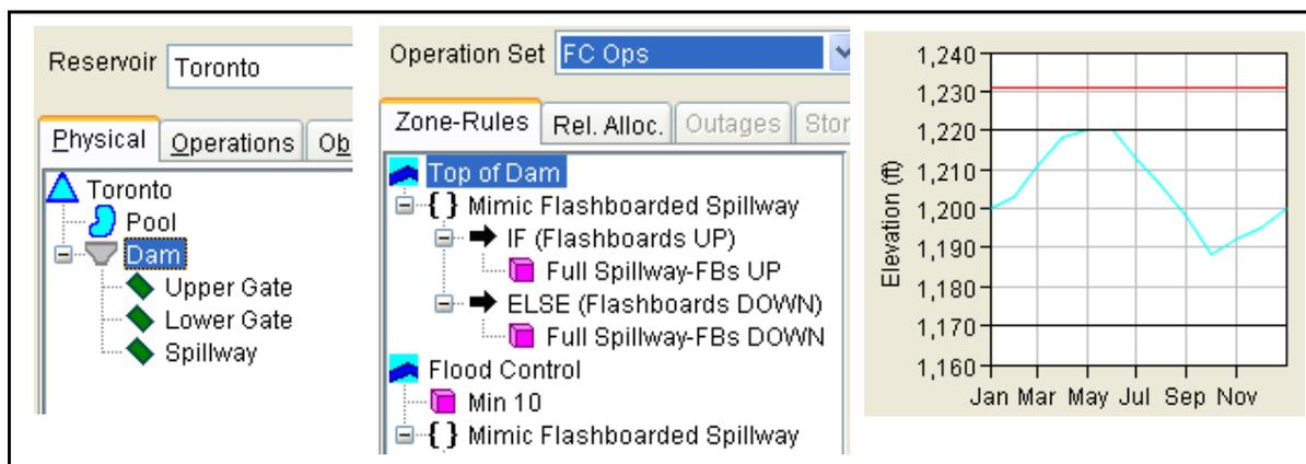
Figure 4.29 Toronto's Pool and Dam Elements and its "operating" zones
