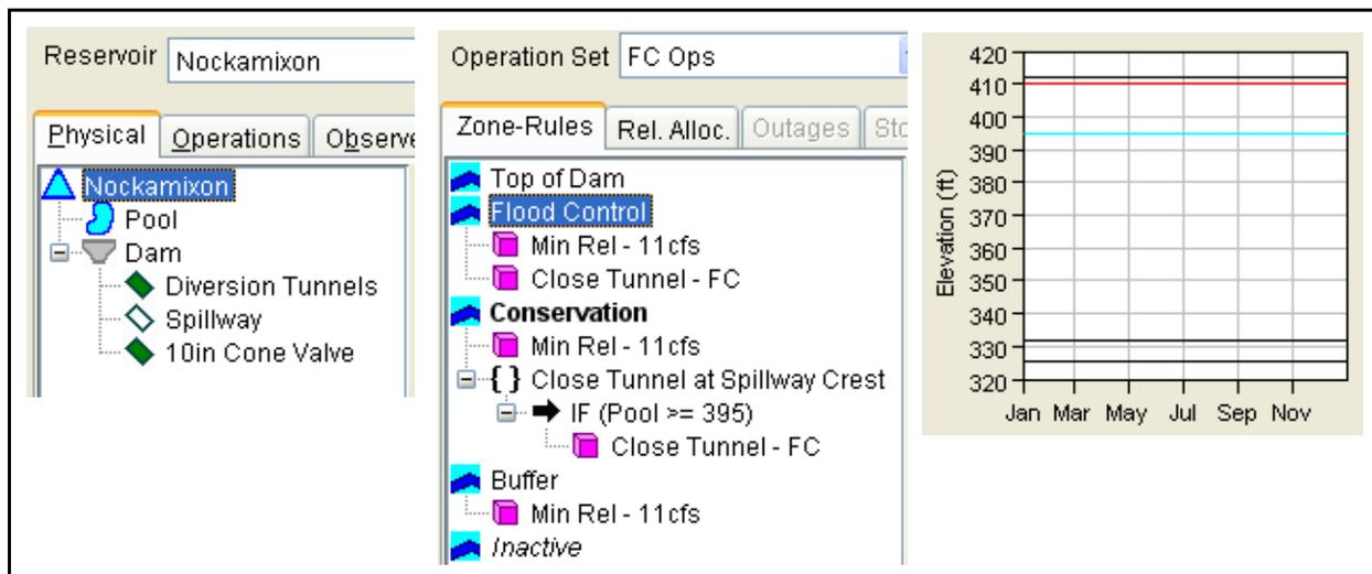
Figure 4.39 Nockamixon's Pool and Dam Elements and its "operating" zones and rules
