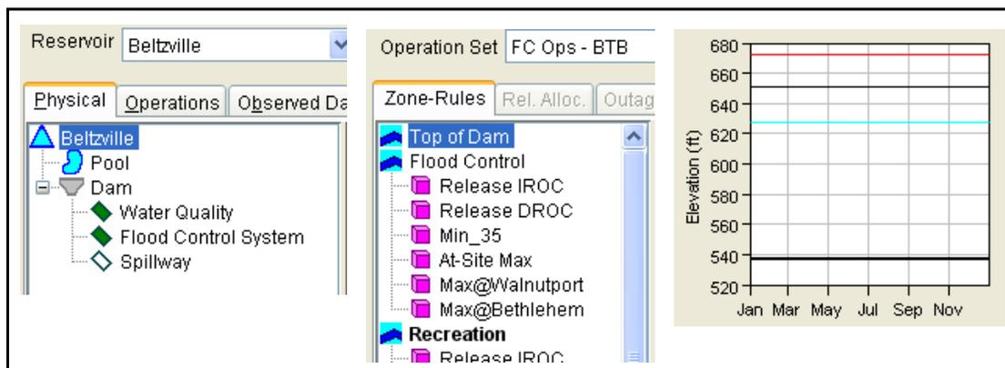
**Figure 4.35** Beltzville's Pool and Dam Elements and its "operating zones" and rules
