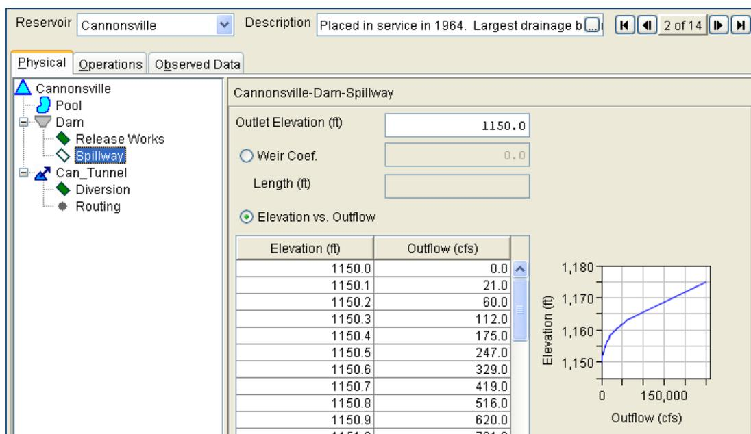
Figure 4.13 Cannonsville – Spillway
