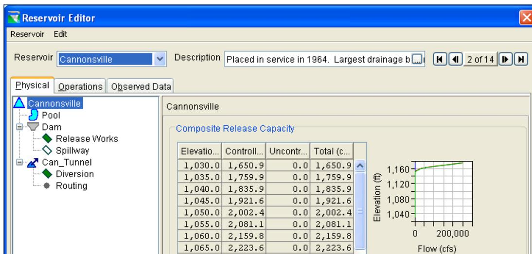
Figure 4.9 Cannonsville – Physical Element Tree and Composite Outlet Capacity Table
