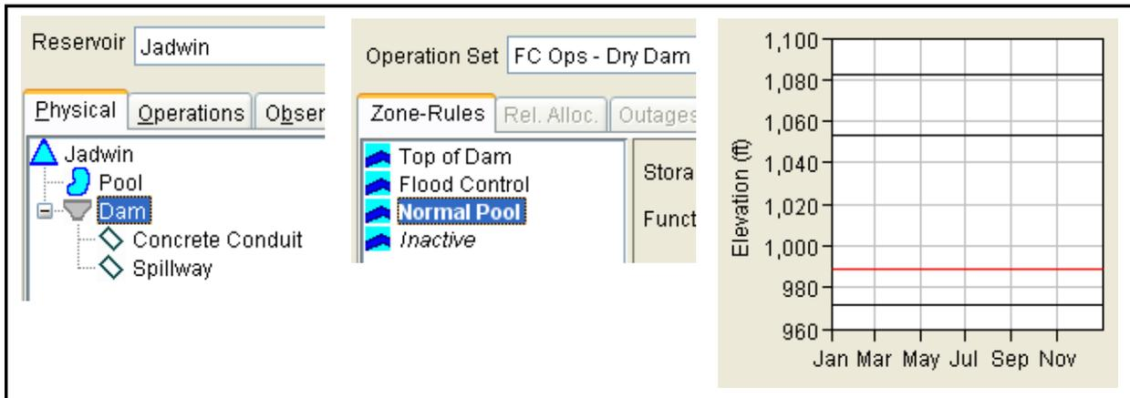
Figure 4.25 Jadwin's Pool and Dam Elements and its "operating" zones
