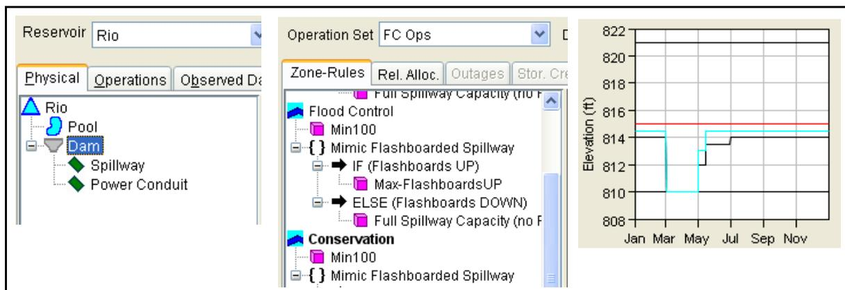
Figure 4.32 Rio's Pool and Dam Elements and its operating zones & rules
