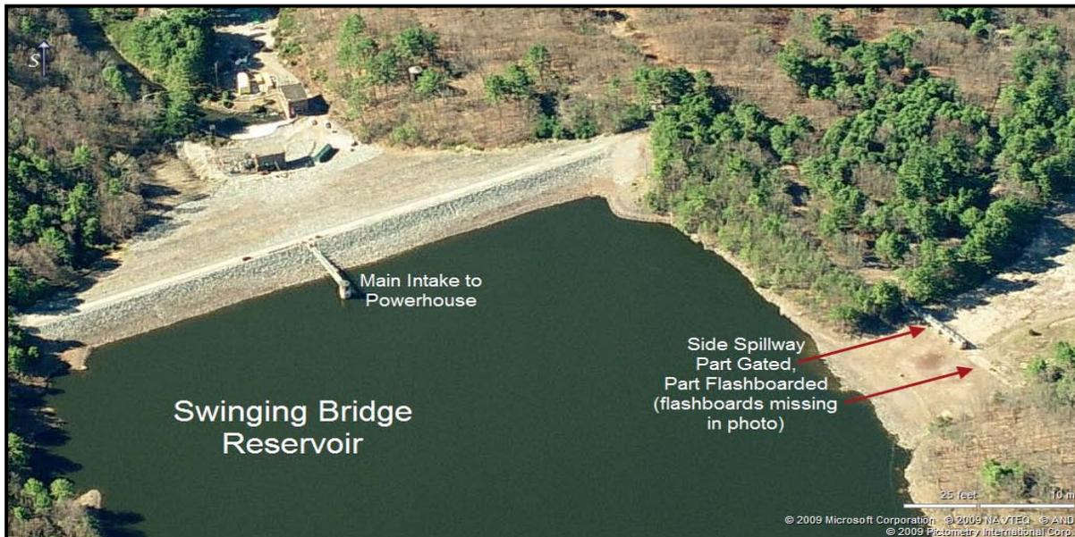
**Figure 4.30** Swinging Bridge Reservoir
