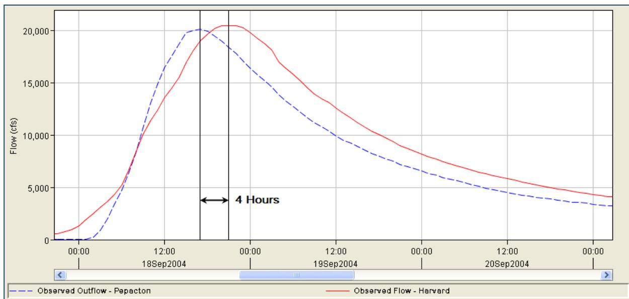
**Figure 4.4** Observed Releases from Pepacton Reservoir and Observed Discharge at Harvard
