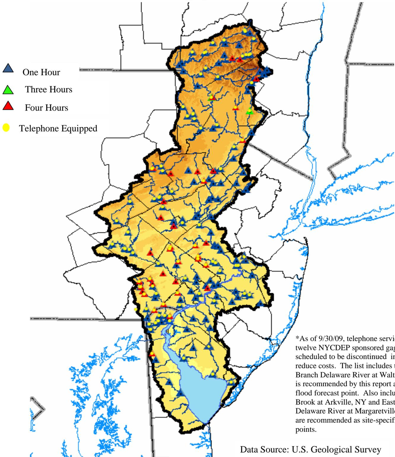
Note: The reporting interval is the time between reports to the satellite. Flow and stage data is generally collected at 15 minute intervals. Telephone equipped gages can be polled to provide stage information as needed during storm events.
