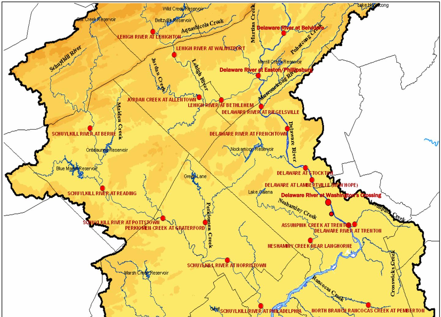
**Note:** The Delaware River at Washington's Crossing, NJ/PA will not be equipped with real time stage monitoring until completion of bridge construction work in 2010. The site is included on this map because it currently serves as a flood forecast point. Flood stages are forecast by the MARFC using a stage vs. stage rating referenced to the real time gage for the Delaware River at Trenton, NJ, and manual wire weight gage measurements conducted by the Delaware River Joint Toll Bridge Commission.
