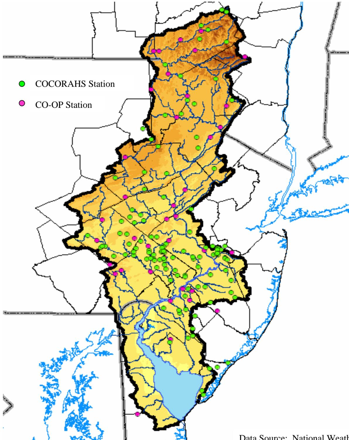
**Figure A-4: Location Precipitation Gages Operated by U.S. Army Corps of Engineers, New York City DEP, U.S. Geological Survey, and the State of Delaware (DEOS) and Used in NWS Forecasting**
