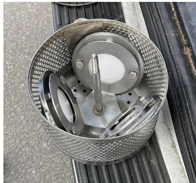
Figure 4 POCIS, membranes, rings inside a sampling canister
