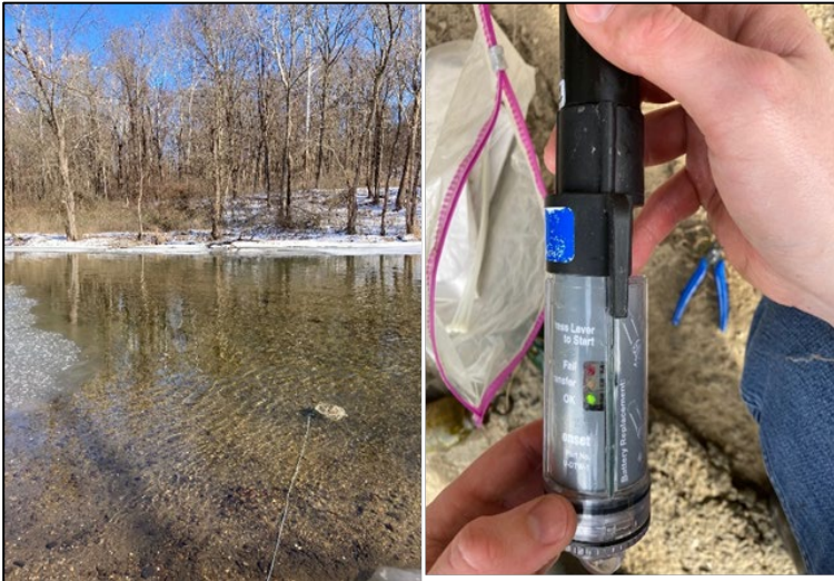
Continuous conductivity (HOBOT® U24) deployment (left), and logger maintenance and data offload (right).
