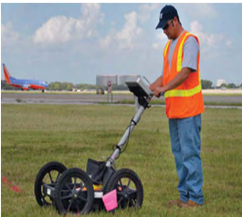
Ground Penetrating Radar
