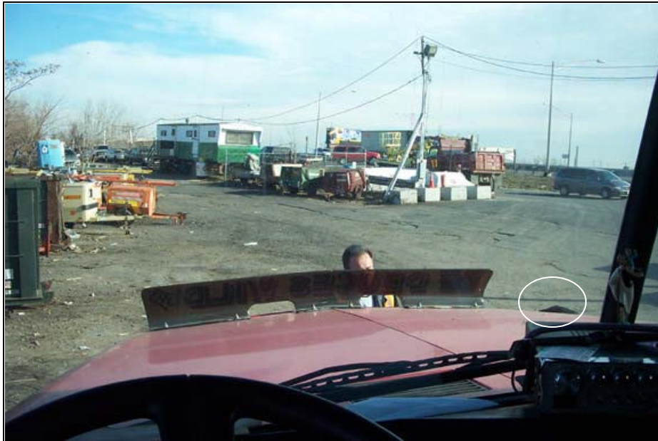
Driver's field of view inside of tanker truck Note pedestrians in front of and directly to the right of bug shield
