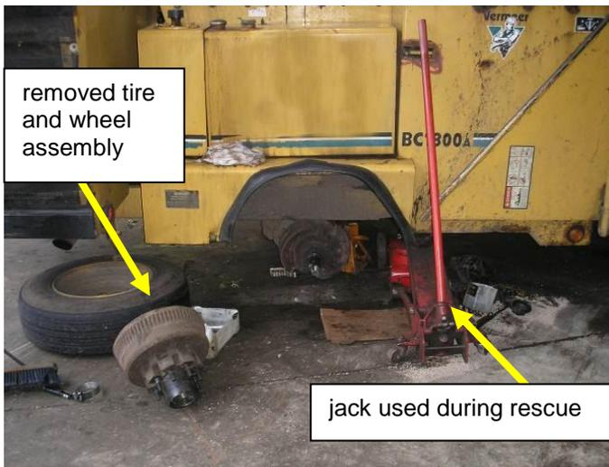
removed tire and wheel assembly
