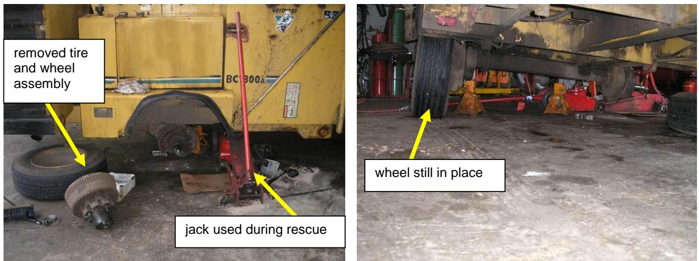
**FIGURE 3.** Air/hydraulic jack used to lift wood chipper.
