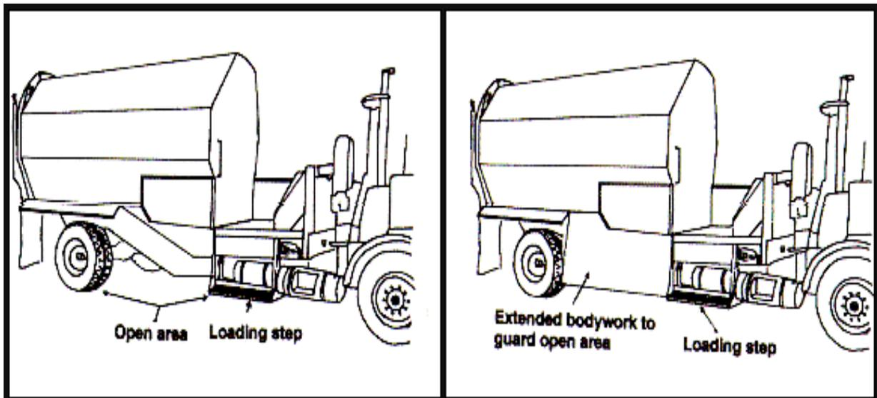
NIOSH illustrations showing the guarding of the open area between the loading step and rear wheels
