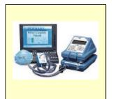
Quantitative: Computerized means of detecting face seal leakage
