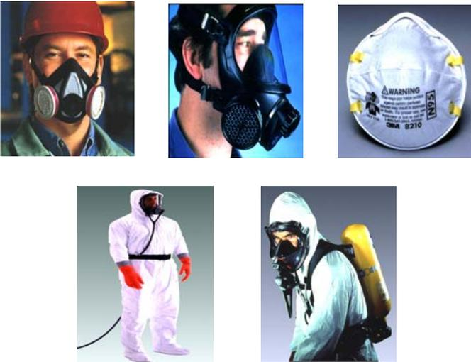
There are two major classes of respirators: (1) air-purifying to remove contaminants from the air, and (2) atmosphere-supplying to provide clean, breathable air from an uncontaminated source. As a general rule, the latter-type respirator is used for more hazardous exposures.
