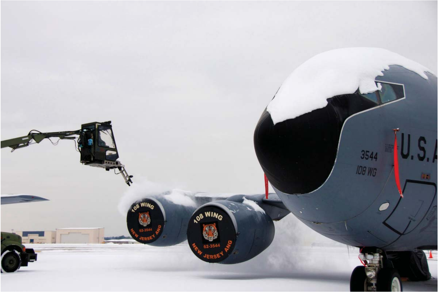
Above: Senior Airman Ryan Galante from the 108th Maintenance Squadron, 108th Wing, blows an over-night snowfall from a KC-135R Stratotanker using a forced air deicing system from the enclosed operator cabin at the end of the 42-foot boom of the GL 1800 deicer truck at Joint Base McGuire-Dix-Lakehurst, N.J.,
