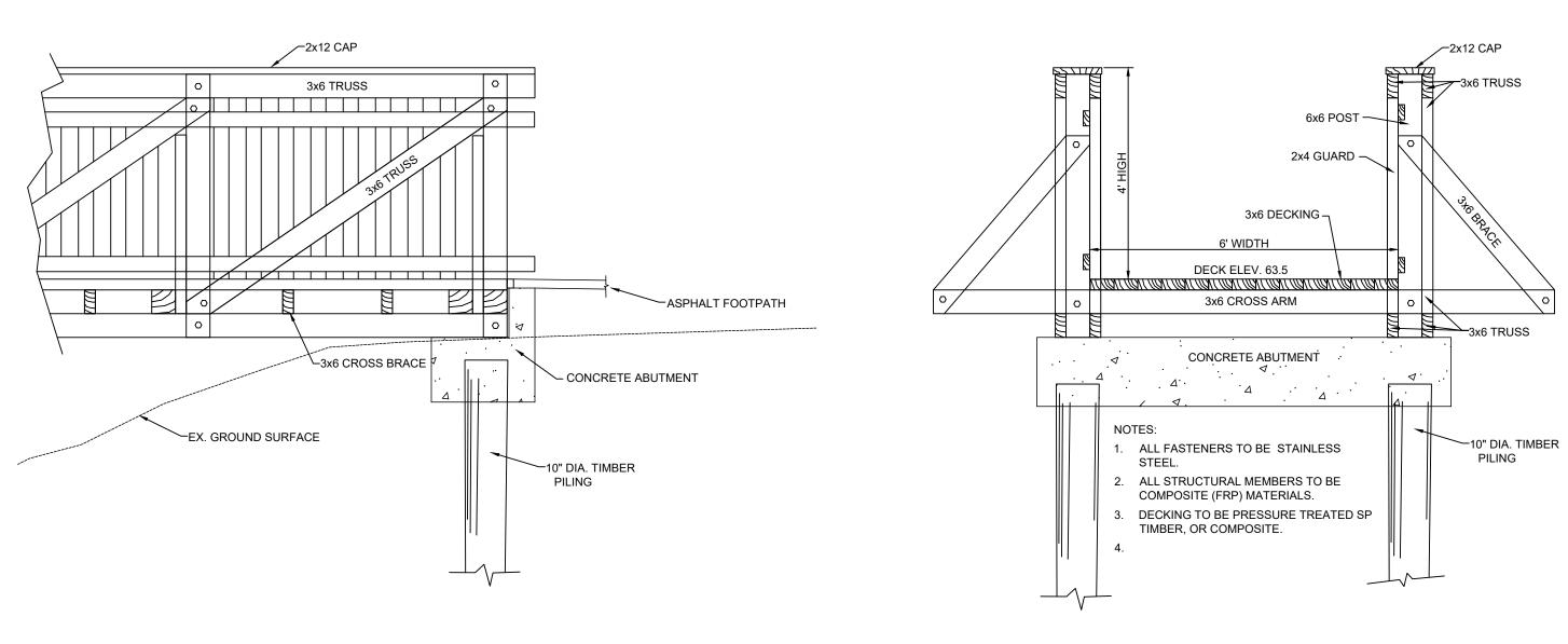
TIMBER TRUSS FOOTBRIDGE SCHEMATIC CROSS SECTION
