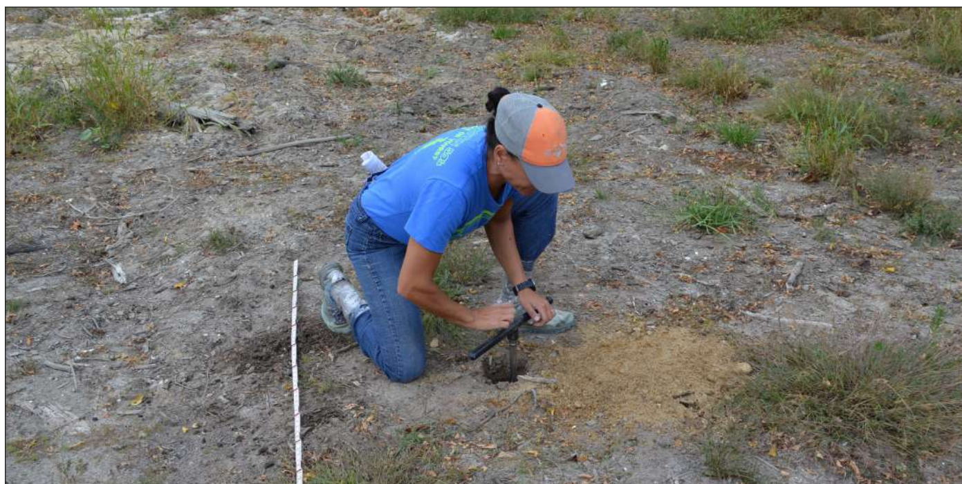
Above: Branwen Ellis, a Pinelands Commission Environmental Specialist, conducting soil borings in the field as part of the agency’s review of a development application in the Pinelands. Photo/Paul Leakan
