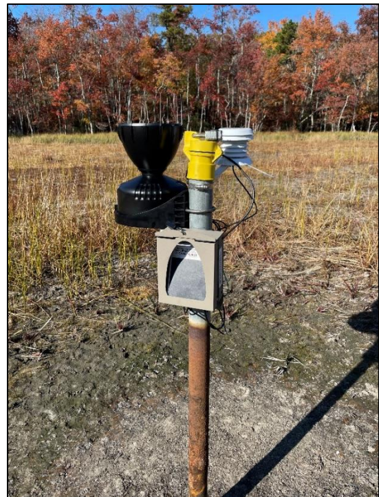
Above: This solar-powered weather station was installed in a continuous monitoring pond that currently has no standing water due to drought conditions.
