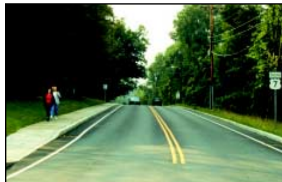
Figure 3.3.1.4: Typical section with narrow shoulder entering town.
