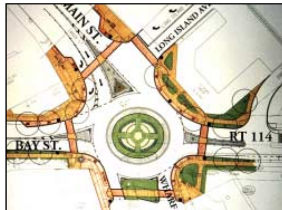
Figure 3.3.3.10: Proposed roundabout in Sag Harbor Village Center.
