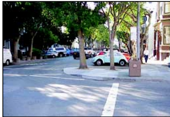
Figure 2.14: Curb extension with space for trees, San Francisco, California.
