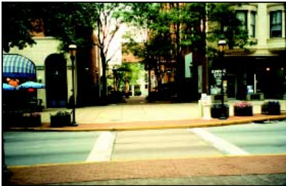
Figure 3.3.6.20: Mid-block crossing aligned with mid-block passage.
