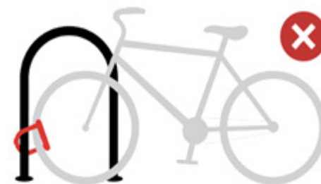
U-Lock secures front wheel only, leaving rest of bicycle vulnerable to theft.
