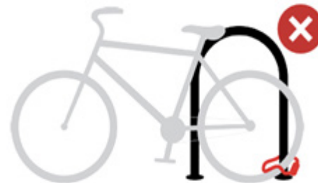
Cable lock secures rear wheel only, leaving rest of bicycle vulnerable to theft.
