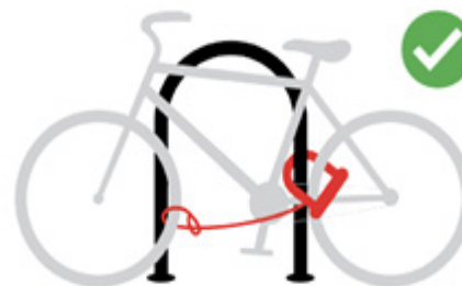
U-Lock secures rear wheel and frame, with additional cable to secure front wheel.
