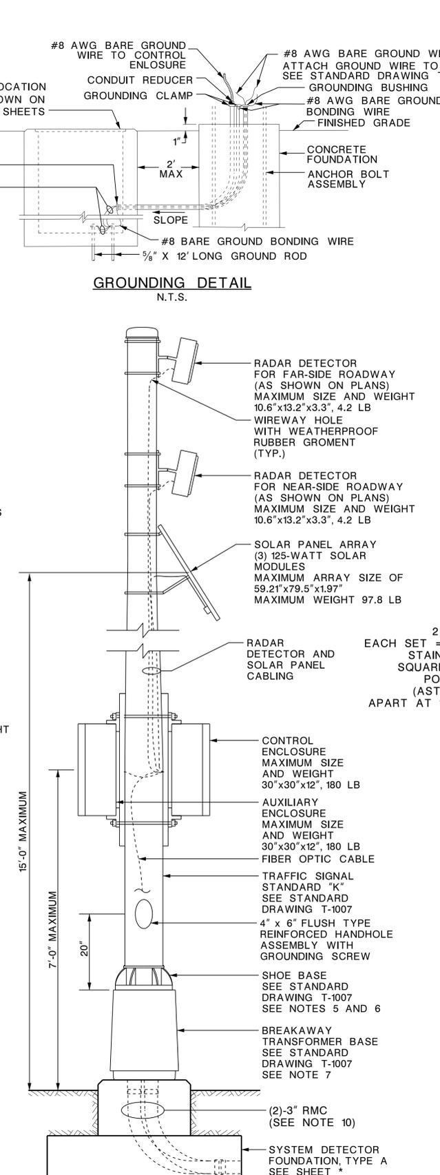
**SYSTEM DETECTION, TYPE RADAR AND SOLAR POWER SYSTEM, TYPE A ON TRAFFIC SIGNAL STANDARD "K"**
