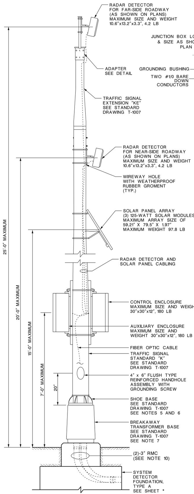
**SYSTEM DETECTORS, TYPE RADAR AND SOLAR POWER SYSTEM, TYPE A ON TRAFFIC SIGNAL STANDARD "K" WITH "KE" EXTENSION**
