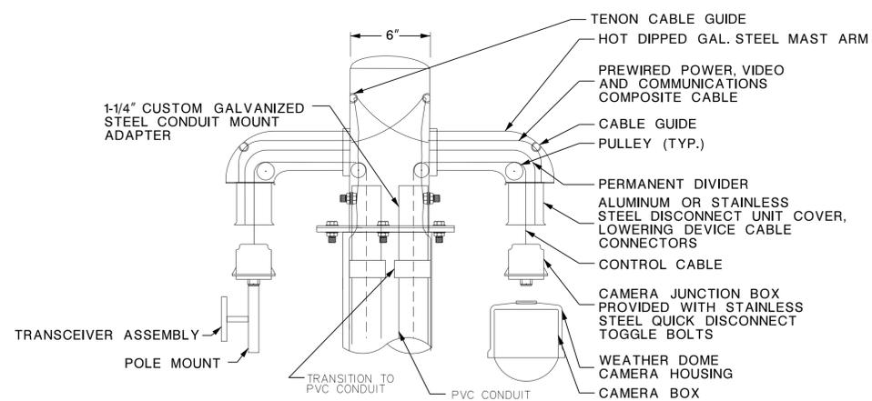
**DUAL LOWERING DEVICE ASSEMBLY DETAIL**
