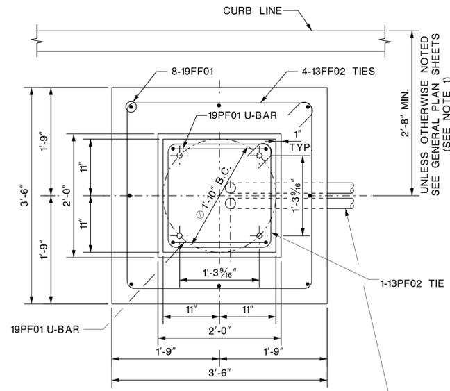
SEE GENERAL PLAN SHEETS FOR NUMBER & SIZE OF CONDUITS REQUIRED AND POSITION OR DIRECTION OF CONDUIT RUN.
