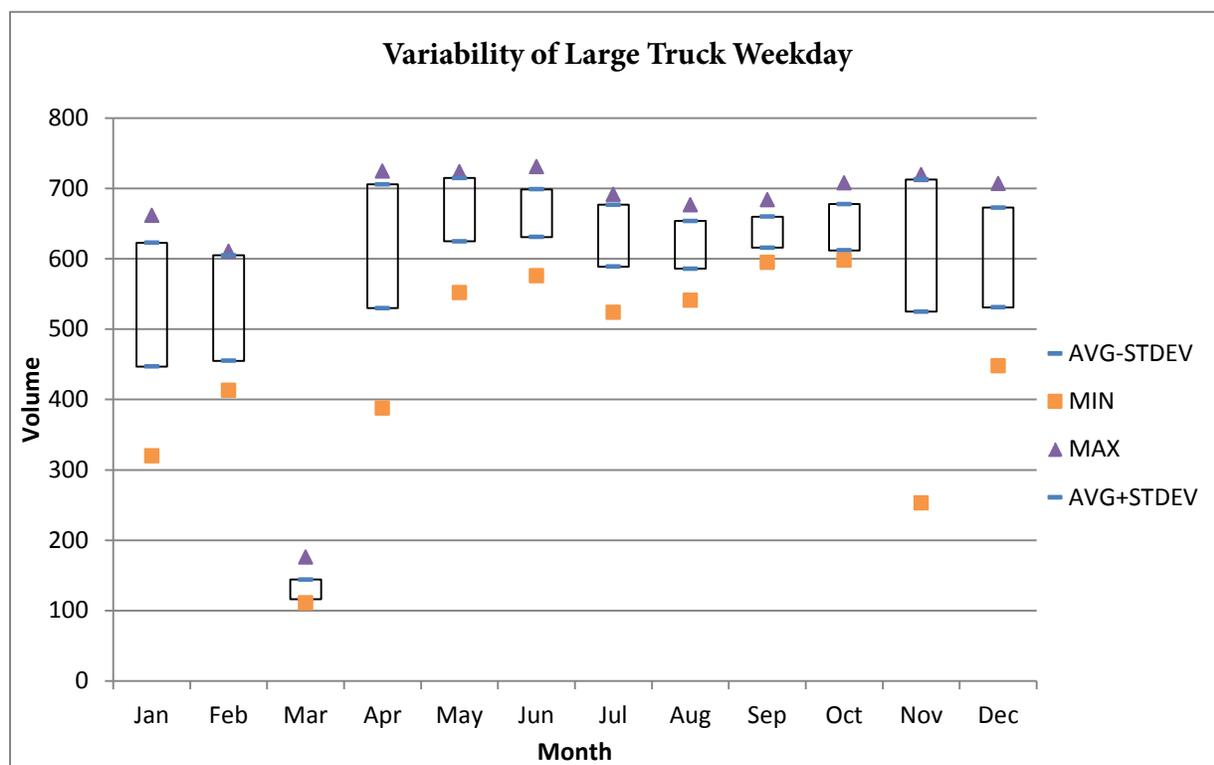
**Figure 100.** Variability of Large Truck Volume at Northbound NJ 31, MP 13.0 (2011)
