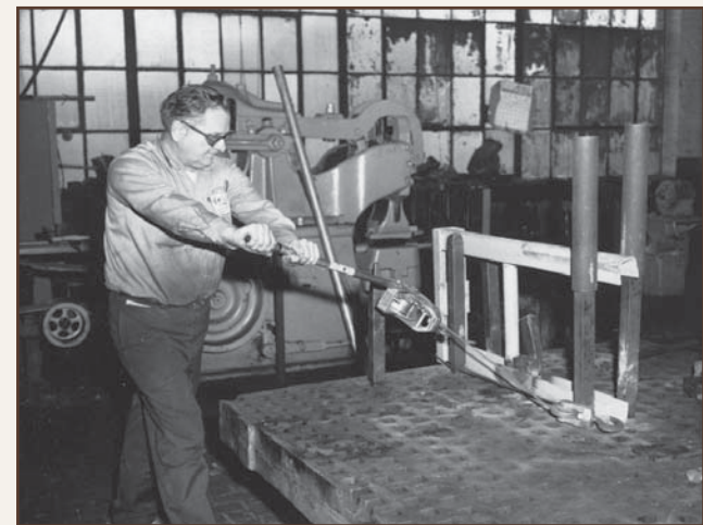
Joseph J. Odas, blacksmith, Straightening Part of a Snow-Plow Frame, 1972.
