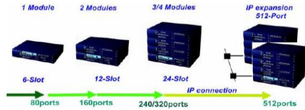
Figure 12 UHNERGE SV8100 CHS2U-US 19" Chassis Expansion
