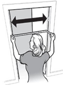
This measurement equals the clear open width of the door, which is typically less than the width of
