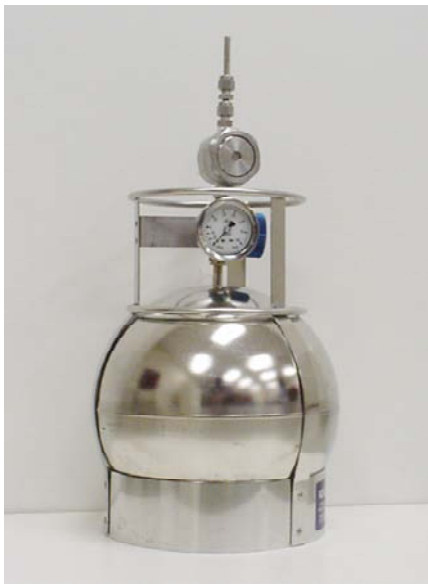
An evacuated air testing canister. The pressure inside the canister is initially set lower than the indoor air, causing air to flow into the canister when the valve is opened.
